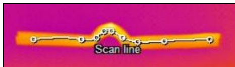
Scan line with multiple points as spline
